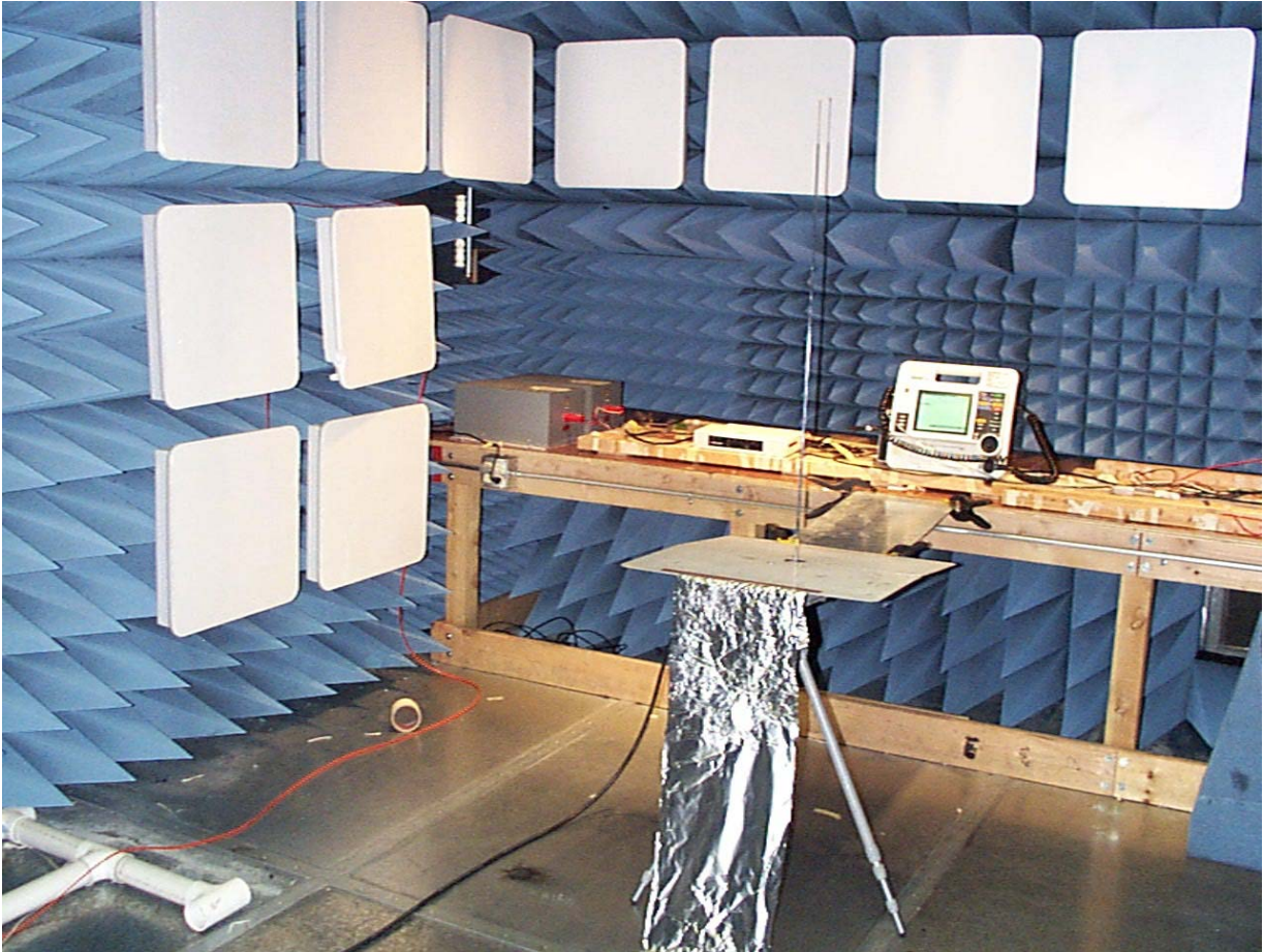
Figure 3 – CKC Rod antenna setup and experiment
